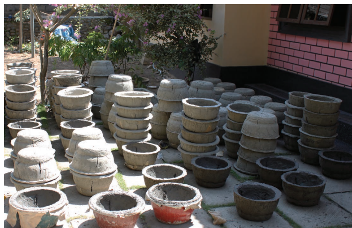
Artificial reef structures ready for installation on the reef. Photo: James Frey
